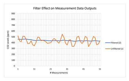
The graph above shows the effects of the filter on the  $CO_2$  measurement data (Z or z). The unfiltered output is shown in orange and the filtered output shown in blue.
