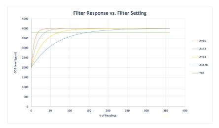
The graph above shows the effect of the filter on response times. Increasing the filter setting increases the measurement output response time.  $T_{90}$  is the time to 90% of reading. The SprintIR<sup>®</sup>-R takes 50 readings per second. The flow rate was set at 0.21/min.
